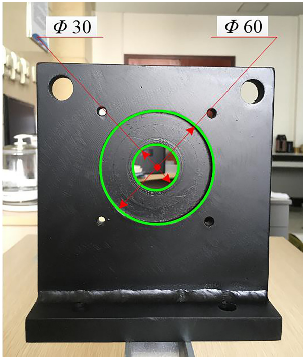
Fig. 8 The workpiece with concentric circles.
