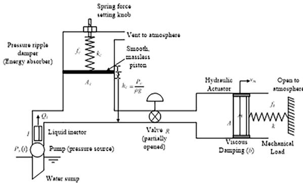
Fig. 4 Water pumping system for a hydraulic actuator.
