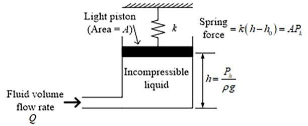
Fig. 1 Two series capacitors in a fluid-mechanical device.
