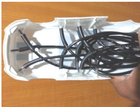
Fig.3 Pressure Tapping Connection Tubes Fitted to the Car
