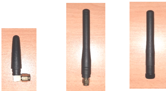
Fig.2 900MHz, 1800MHz, 2400MHz Rubber Duck Antennas
