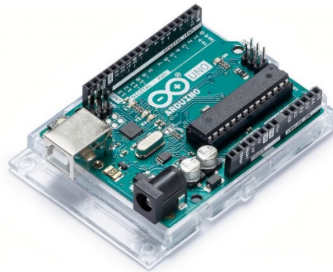
Fig.1 ARDUINO Uno r3 Physical Map
