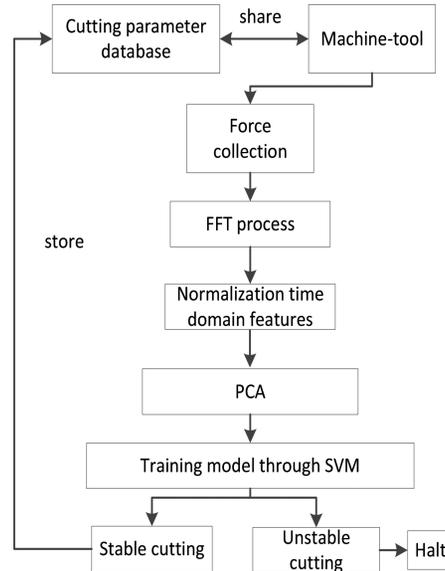
Fig. 1 The Flowchart of Milling Chatter Diagnosis.
